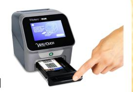
While strip test develops, enter the sample ID into Vertu TOUCH reader.
