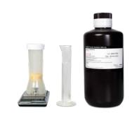
Set Vertu PREP mixer for 30 seconds. Push down and twist to lock the tube on the mixer. The mixer will start automatically. Filter the extract into a V-Filter w/Cup for no more than 5 minutes.
