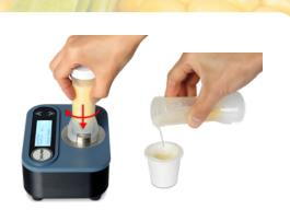
During incubation, enter the sample ID. Fully insert the T2/HT2-V strip into the Vertu TOUCH (the round opening in first), then press [Start Measurement].
