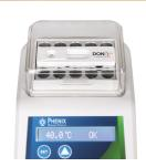
Transfer 100 µL diluted extract to the DON-V strip by dropping vertically into the circular opening, close the incubator lid, and develop exactly 5 minutes.
