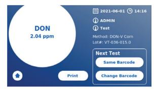
If display shows >Range, press [Change barcode] to scan or select the High Range barcode DON-V G for wheat or DON-V I for corn for the lot being used. Transfer 100 µL of diluted extract from Step 4 into a new strip test vial. Add 1000 µL of AQUA solution. Mix well by vortexing. Repeat steps 5–8, using this twice diluted extract.
