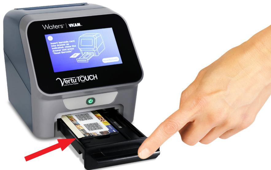
Make sure, the barcode card is positioned on the left upper side of the drawer. Your drawer will contain a small bar to give you an edge for the card which shall be placed above (see red arrow).
