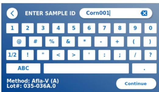
The [Continue] button appears if at least one number or one character is entered. Pressing [Continue] leads to the final screen before the measurement starts and prompts the user to insert the test strip/cassette into the drawer.
