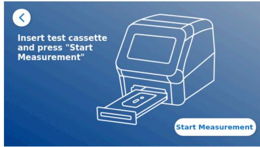
Insert the test cassette now into the drawer. Ensure to have the test cassette placed in the correct orientation, round circle in first, close the drawer and press **[Start Measurement]** immediately.
