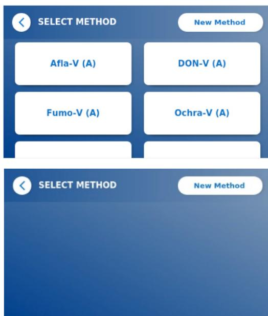
The menu shows an overview of all scanned test barcodes. Via the search field, filtering for a set of dedicated test methods can be applied. To import a new test method, press **[New Method]**. A window prompts you to insert now a barcode card, which contains the test method to be imported.
