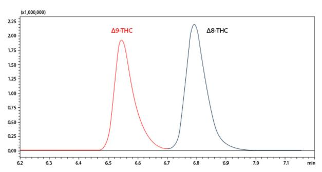
Figure 2. Zoomed in chromatogram of 50 ng/mL extracted blood sample showing separation of THC isomers
