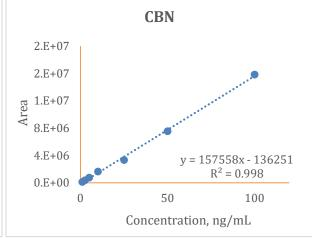
**Figure 3.** 7-point solvent calibration curve for all analytes with linear equation and  $R^2$  value. [1, 2.5, 5, 10, 25, 50, 100 ng/mL]
