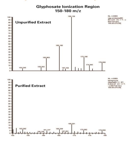
Vegetation samples were infused onto an Ion Trap LC/MS in full-scan mode for an average of 30 seconds pre and post clean-up using UCT's Glyphosate Purification Cartridge. Background matrix that can lead to significant ion suppression and compete with glyphosate and glufosinate during analysis were significantly reduced following clean-up.
