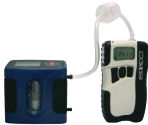
Calibration train with sample medium in line
