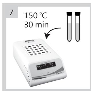
Put the vials into CR 25 reactor then start to countdown from 30 mins at 150°C.
