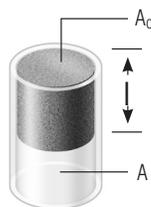
With Gastec's dual layer design, the diffusional cross section area (A) is much larger than the analyzer cross section area (A<sub>0</sub>).
