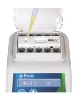
Insert the DON-V strip into the Vertu. Press the center key to take a reading. To print, use the arrow keys to move the cursor to "P" and press the center button.
