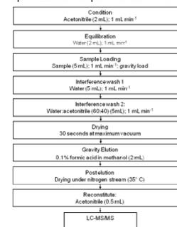
Figure 3: Optimized solid phase extraction procedure
