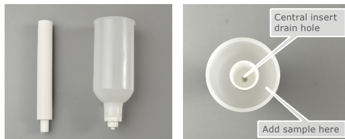
Figure 1: Biotage® Universal Phase Separator. Left: kit form as supplied (2 tubes, 2 screw fittings and 3 inserts), right: assembled.
