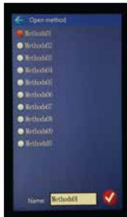
Up to ten pre-set methodologies can be stored in the instrument, easily modified and saved, and can be recalled for repeated use.
