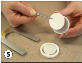
5 Use the forceps accessory to remove the final collection filter and place it in an appropriate container for shipping to a laboratory.
