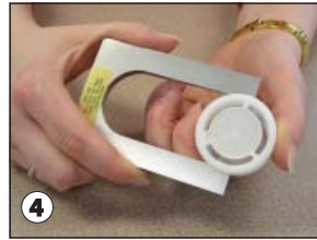
4 Use the cassette opener accessory to separate the two halves.
