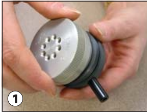
1 Unscrew impactor inlet from exhaust.
