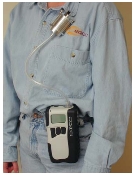
Sioutas Personal Cascade Impactor in Sampling Train.
