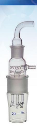
The SKC BioSampler is a bio-aerosol collection device resembling an impinger. The patented design allows high and constant collection efficiency of viable bio-aerosols for sample times of up to eight hours. The BioSampler's three tangential nozzles act as critical orifices each allowing 4.2l/min ambient air to pass through for a total flow rate of approximately 12.5l/min.
