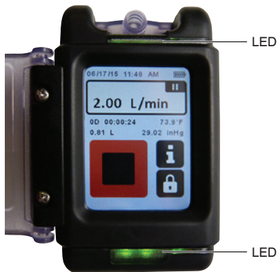
Figure 5. Green, flashing = Pump or schedule running
