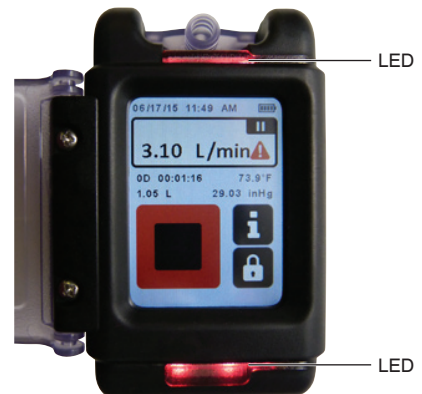
Figure 6. Red, flashing = Flow fault
