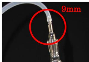
2. Connect the exhaust port on the vacuum pump and the port on the upper part of the condenser.
