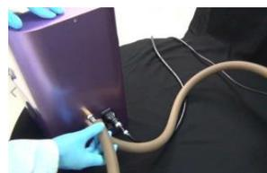
3. Connect the port on the lower part of the condenser and the port on C1 for the circulation hose.
