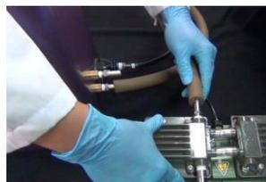
1. Connect the port on C1 for vacuum pump and the suction port on the vacuum pump.
